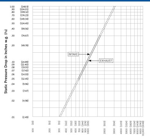
Air Velocity in feet (meters) per minute through Free Area
